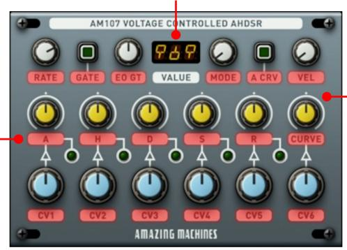
The white dots that circle around the A, H, D, S, R and CURVE knobs are Modulation Indicators, they move away from the knobs indicators depending on how the CV1, CV2, CV3, CV4, CV5 and CV6 Inputs are set.
